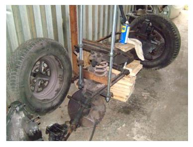
from the gearbox and the rear axle and propshaft came out in one go! For this job I needed a large breaker bar and a lot of elbow grease. Once it was out I went home for a well earned couple of pints!
