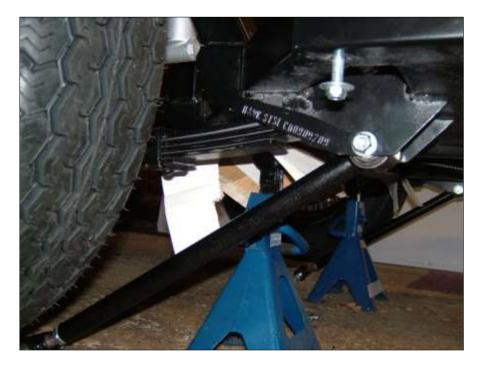
The anti tramp bars mount to the same position as the front mountings for the rear springs but they use the lower set of holes.
