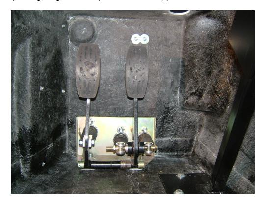
I've got the Hawk pedal rubbers fitted as these are needed for the IVA.
