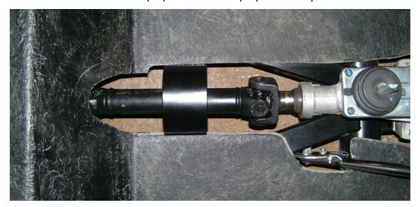
It's important to remember that the rear axle will move up and down so it's best to leave some room! There's a decent sheet of marine ply laminated into the floor of the hawk body shell, so a good jigsaw blade is needed!
