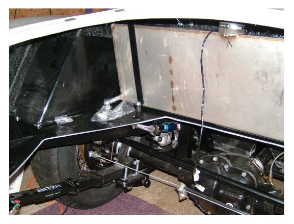
I cut and fitted some heater hose under the tank straps where they attach to the boot floor as it says in the build manual. The 3/8" ID hose I had was perfect for that.
