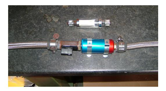
The filter came with two mounting spring clips and used the old hose and banjo connections.
