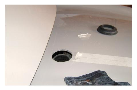
I then had to cut down the filler cap adaptor (as it was too long), fit the grommet, fit the filler pipe and drop in the fuel cap and adaptor.
