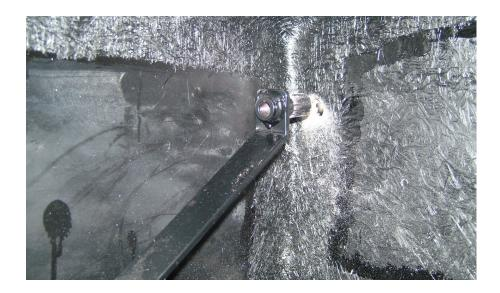
The bolts for these straps are included and the other end fixing utilises some bolts that are already used to bolt the body to the chassis in the boot place the tension straps in place and you can see which ones are used. These bolts need to be removed as the tabs on the straps need to be drilled to accept these bolts.
