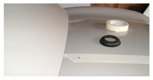
I found the centre line of the car which coincided with the mark in the gel coat for the filler cap and drilled a pilot hole.
