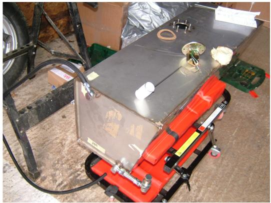
This gives me a sender that works freely and when it is at the bottom (i.e. fuel tank empty) this still leaves a couple of gallon of petrol in the bottom of the tank.
