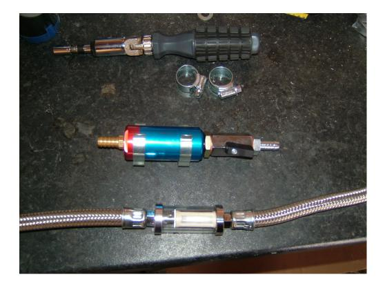
One option is to fit a "shatterproof" aluminium filter and whilst I was at it, I fitted a tap to isolate the fuel tank. Just in case I needed to change the fuel filter.
