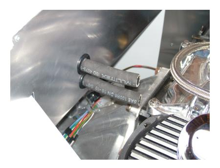
I'd always planned to route the coolant pipes using stainless steel and I cut bent and welded two lengths of 5/8 tube to suit.
