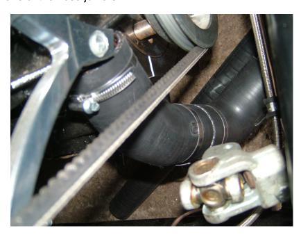
The flexible 1 mtr straight lengths have an impregnated wire helix to stop the hose from kinking or collapsing. They are cut to the required length.
