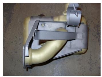
I already knew that it would require a bit of modifying as this version of header tank connects up directly to the block, similar to the 427 cobras, and I wouldn't be using this option. The mounting bracket would need replacing as it's a bit of a squeeze under the Hawk bonnet but we'll get it sorted one way or another. The tank looked as if it had been through a couple of battles and was a tad dented but we'll sort that out too.
