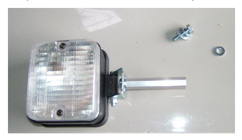
I cut a short length and drilled and tapped each end.
