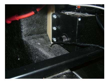
The handbrake switch is a small normally closed push button switch available from RS.
