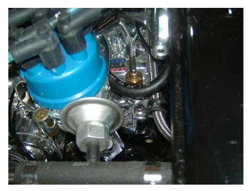
The oil temp is best taken from the sump. I'd already fitted a suitable bulkhead fitting in the sump when I assembled the engine (all those months ago!). It was now time to make the connection.
