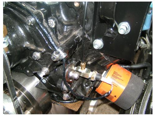
I then tried to route the pipes neatly. The coils in the pipes between the engine and bulkhead were to take up the excess length and also to dampen any vibration. The other end of the oil pressure pipe could then be connected to the pile of spaghetti that is the rear of the dash board. The pipe tightens up on the respective fitting on the back of the Oil pressure gauge using the fibre washers provided in the pipe connection kit which can be supplied by the gauge supplier.
