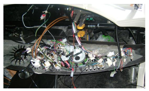
This picture also shows the conduit that sheaths the rear harness, which is laid from the boot area under the driver's door and up the scuttle frame leg. It also shows the connections for the ammeter (the brown heavy gauge wires). I've made the all the connections to the dash harness long enough to make it easier for the dash to be removed, but not too long as to make it a tight fit behind the dash when it's installed.
