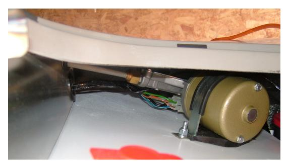
I then made up the plug connection for the nearside side repeater and plugged it into the harness. The excess could then be cable tied into a loop to neaten it up a bit. Whilst I was working down this side I fitted a clamp to hold the battery in place.
