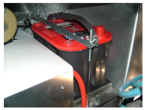
Whilst the battery tray that Hawk supply is nice and the battery fits into it a treat and stops it sliding round, I'd prefer to have a bit of extra security here. As the battery was now secured, the battery cable could be connected to the positive terminal to the battery ensuring first that the isolation switch was off and the key was removed. This would be switched live when we get round to testing the loom.
