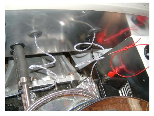
I also drilled another hole for the oil pressure plastic pipe and fitted a suitable grommet for that too.
