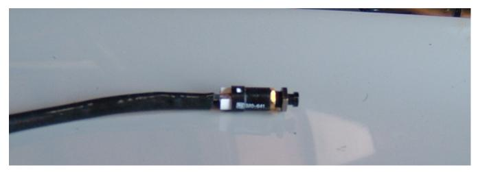
I soldered on some flying leads and fitted some insulated spade connectors. Fitting this, to the handbrake, is another extremely fiddly job that is much better installed with either the body off or, better still, fitted to the handbrake before it is bolted to the chassis.
