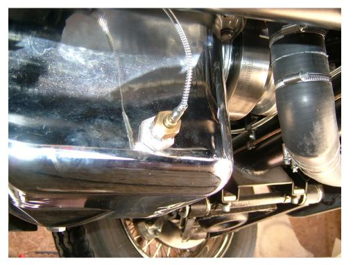
The final mechanical connection to be made was the oil pressure. I took this from the same position as the oil pressure warning light switch which on the Ford engine is by the fuel pump blanking plate.
