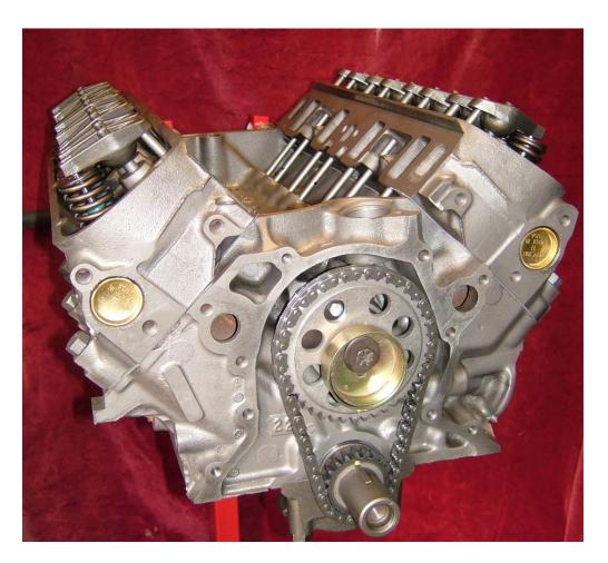
It had been totally stripped, blasted, cleaned and tested for cracks. It had then been checked, balanced and reassembled.
