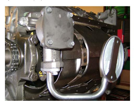
After the oil pump I had to think of the sump pan. I ordered a nice chrome pan and thanks to my research I found out that the oil temperature is best measured when the oil is in the sump. If you try and measure it in the engine block then you generally measure the block temperature. This doesn't give the required warning of too high oil temperature.
