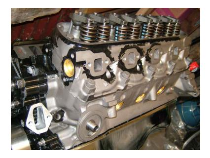
Then I fitted the Intake manifold using the correct gaskets and Gasgacinch. The key is also to add some RTV sealant around the water passage holes. The "How to Rebuild a Small Block Ford Engine" book explains this in detail.
