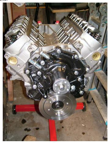
I decided that I would fit a windage tray, recommended in all of the books this allows the oil in the sump to flow from the crankshaft in a more controlled manner and reduces the foaming of the oil due to aeration. To fit this you need to exchange four of the bearing block mounting bolts for special bolts with integral female threads to allow the windage tray mounting bolts to screw into them.
