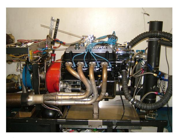
After 2 coughs it ran up like a dream. We ran it for ½ hour at 2300 RPM to bed the cam in and then wound it up to 5200rpm. After some adjustments it made 210HP and had a nice flat torque curve of 275ft/lb from 1000 RPM up to 4500RPM, perfect for a street car engine.
