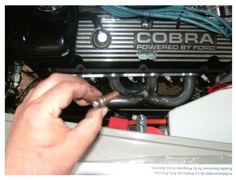
I smeared exhaust assembly paste on all of the joints and assembled the exhaust.
