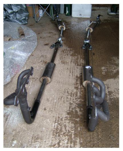
The back part of the exhaust comes with all the brackets, rubber bobbins and clamps required and I had the header bolts in the 289 engine bolt kit that I had and the header gaskets were in the gasket kit. The only other things needed, in addition to what was already supplied, to fit the exhaust were a couple of M10 bolts, nuts and washers (to mount the centre brackets to the chassis), and some exhaust assembly paste.
