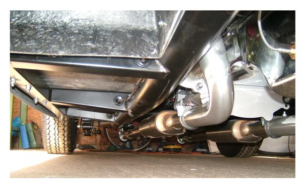
I tightened up all the clamps and made sure that the bobbins and brackets were tight.
