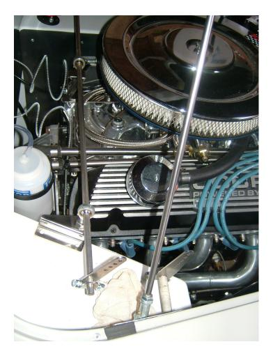
For the carb end I made a connecting arm using the aluminium hexagonal bar and the rose joints supplied in the kit.
