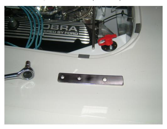
This could then be bolted onto the inlet manifold and using the angled bracket that Gerry supplied (I just polished it) this makes a nice support for the throttle linkage at the engine end.
