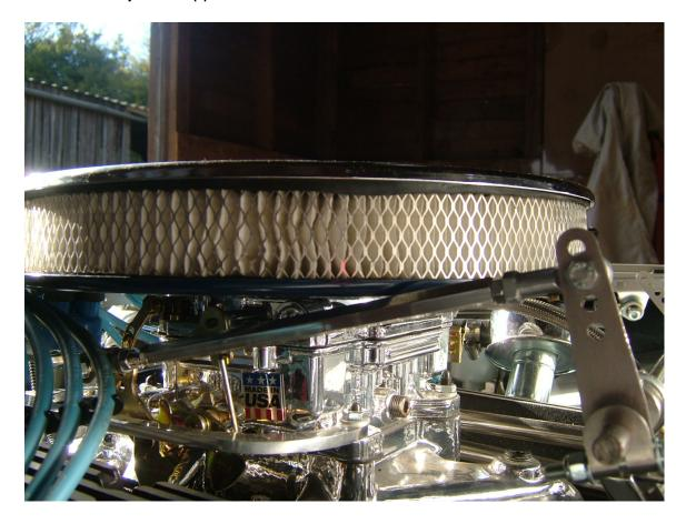
On the accelerator pedal end I fitted the stainless actuating arms and the longer length ½" diameter accelerator pedal bar. After connecting the linkage arms, I tried it out.
