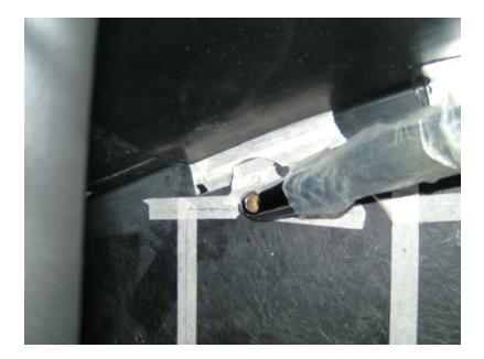
Last thing up on this episode was to bleed the clutch and brakes. I've already got a small compressor so I bought a vacuum bleed kit to use. Never used one before but they are quite simple. Rather than pumping the pedal for ages, the kit uses compressed air to create a vacuum which sucks the brake fluid through. The theory is that when the air bubbles stop being pulled through and it is pure brake fluid, then the system is fully bled.
