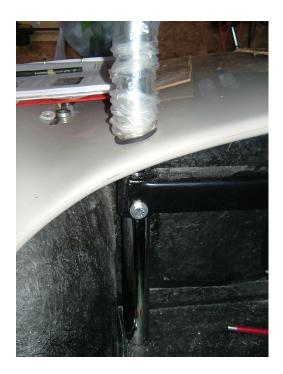
I could then drill the two 7/16" clearance holes (as described in the manual) to bolt the hoop to the SVA frame. The one side uses the bolt that fixes the SVA frame to the straps in the boot and the other side just needs an additional bolt.
