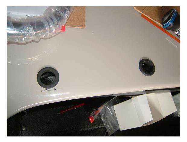
The next stage was to drill the hole to enable the longer leg of the bar to be bolted to the chassis. The hole through the chassis is already present but it's a pig to get at. The best way that I found was to drill a clearance hole, from above, in the GRP floor that lines up with the hole beneath. To find the location I marked around the roll bar where is meets the floor, measured and drilled.
