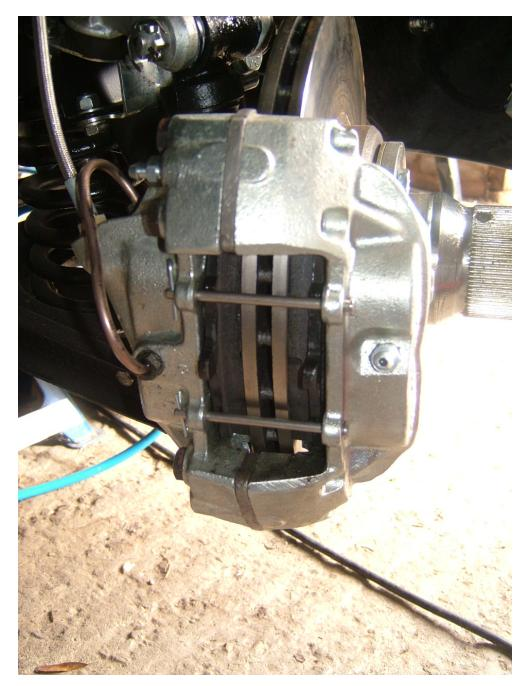
The front calipers took a good couple of hours to bleed. But eventually the pedal was nice and firm. I'd recommend that any work carried out on the brakes be checked by a competent person just to make sure that everything is correct. Cleanliness is extremely important and to ensure that no oils or grease come into contact with the brakes or brake fluid.
