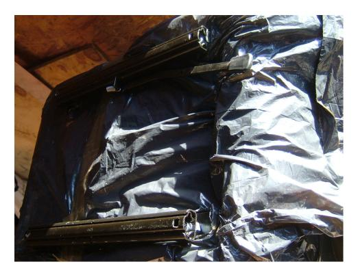
8mm bolts are required as the seat mountings are tapped out to M8. The bolt heads need to be narrow enough to allow the opposing part of the runner to pass over them. The holes on my runners didn't quite line up with the holes in the seats so I had to file the runner holes a bit.
