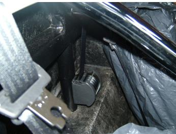
Welded boss on SVA frame where the seat belt reel bolts to.
