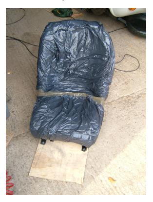
This can be placed into the cockpit and when the correct seat position is found (comfortable, able to reach the pedals avoids the roll bar / handbrake and hood bow locations) you can draw around the protruding part of the board onto the cockpit floor and when the board is removed from the seats and runners and placed in the same position as per the markings, then the hole positions in the board are the correct locations to drill. However...
