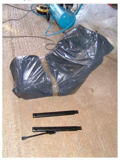
For the seat runners to have sufficient stroke to accommodate mine and my other half's driving position, they need to be spaced off from the seat mounting brackets by about 12-14mm. This equated to a M10 nut and a couple of washers.
