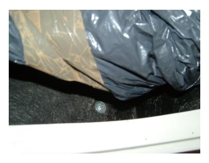
The hole through the floor needs to be enlarged so the 7/16" bolt can be used. I bent a 90 degree bend in two of the brackets supplied with the seat belt kit and, using these, bolted the seatbelt buckles through the floor onto the chassis.
