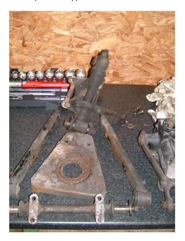
They were all in good condition and just needed a good clean and paint. I tapped up my friend that had the shot blasting equipment and he obliged. After cleaning I noticed that the one wishbone arm on this side was virtually new.
