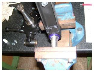
A liberal amount of the provided grease is applied where the bushes come into contact with a metal surface.
