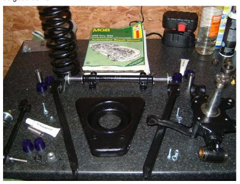
It's just a case of following the instructions with the bushes and using the silicon grease provided in the packet (normal petroleum based grease can react with the polyurethane and is best avoided). Using a vice makes the assembly job really easy.
