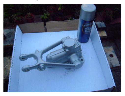
The kingpin and swivel shaft assembly had no play so I cleaned it up and it looked as good as new. The new bushes, nuts, bolts and split pins arrived and I assembled the suspension unit. A large vice is a fantastic investment for removing old bushes and refitting new ones. I bought this vice on eBay for £25.00, money well spent I think.
