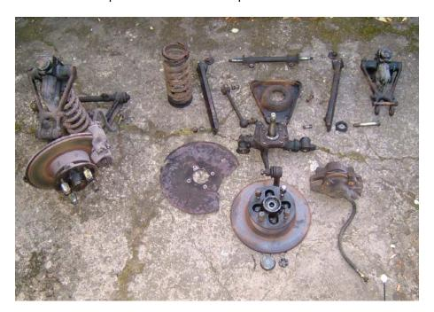
The split pins had had it, the bolts and nuts were all rusted up and the bushes were all shot. I ordered a complete set of these from a local MGB parts supplier. They were very helpful in recommending the required parts and even had a special offer on those that I needed. The spring pan and wishbones were filthy but in good condition and a light shot blast (from a willing friend) and a couple of coats of primer and good enamel and they came up great.
