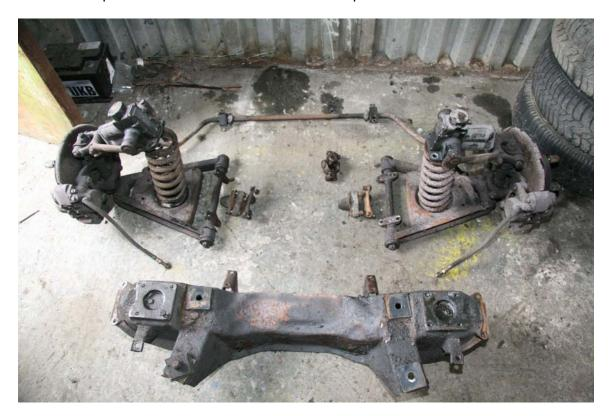
The main suspension cross member isn't required as these attachment points are all included in the Hawk 289 chassis so this was discarded. I decided to refurbish one half of the front suspension first and then the other. Despite having by this time a well thumbed Haynes MGB manual and Practical Classics MGB renovation manual I'd at least have a mirrored completely assembled unit that would give me some indication on how it all went back together.
