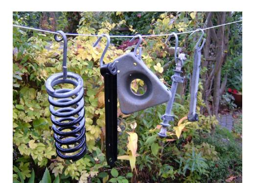
The Armstrong shock absorber was in good condition and only needed a clean up with a wire brush and a coat of paint.
