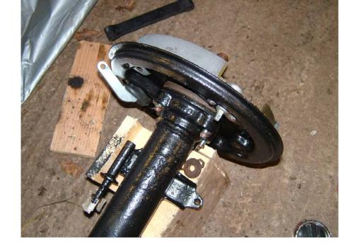
Plenty of copper slip on the bolts and nuts.
