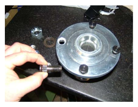
The hubs are bolted on with the castellated nuts and the locking taper.
