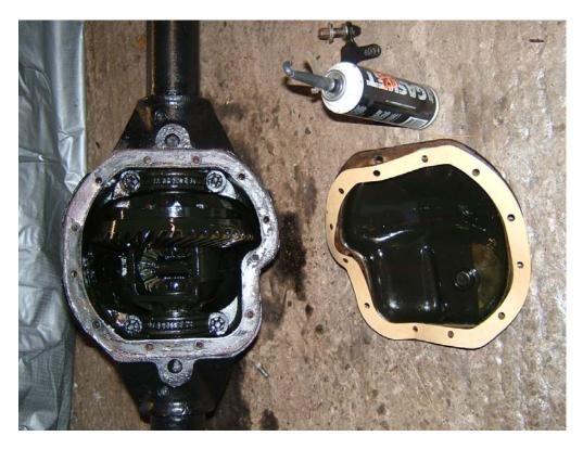
I used the permatex gasket sealant on one side of the gasket. I fitted the cover with new zinc plated bolts and it really looked good.
