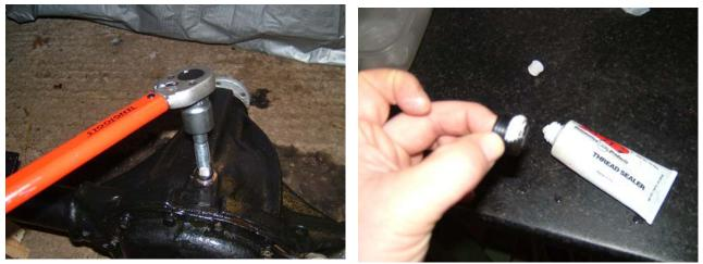
The new plugs were fitted with a smear of ARP thread sealer. I used this on the engine assembly too.
