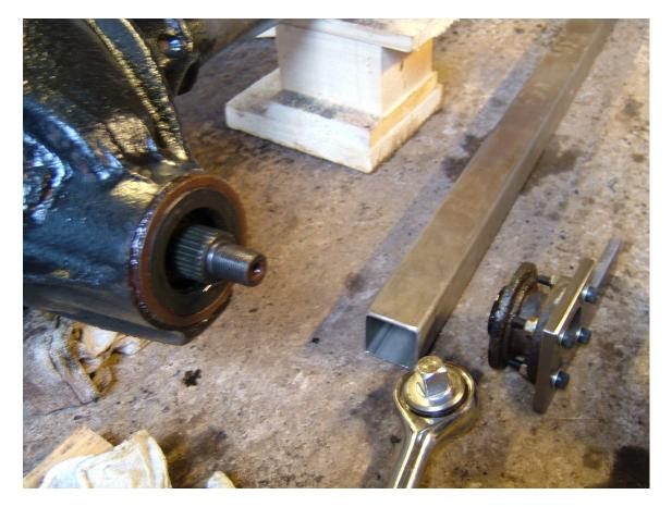
It was then a simple job to lever out the seal, clean out the gunge and tap in a replacement seal with the lip lubricated with gear oil. I then slid the pinion collar back over the shaft and tapped it home with a hammer and block of wood.
