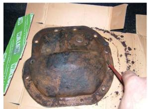
I primed using phosphoric acid solution which is the recommended primer for the paint I was using and applied some paint.
