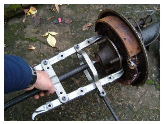
I wound up the pulleys and nothing happened. The jacking bolt got tighter and tighter and then BANG! and the hub was off.
