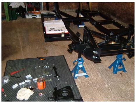
From my experience it's always good to do a dry run with nuts and bolts so you find out if they fit and also work out the correct order for washers (spring and flat). The other thing I decided to do, after stripping an MGB with all of its rusted nuts and bolts and after reading the Hawk build manual, was to use anti seize compound on all of the bolts. This can be a bit messy but I know it'll pay dividends in years to come.
