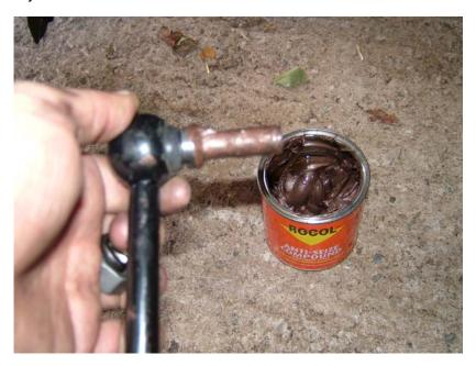
Next up, the Kingpins. Top trunion to the shock absorber first (with bushes well lubricated).
