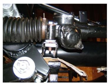
Use the bolts provided in the "Steering rack" bolt pack and some anti seize compound. The bolts pass through the steering rack, through the spacer, through the chassis and into the threaded plates.
