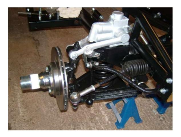
The split pins are fitted next. The holes on my hubs all lined up which made this an easy job.
