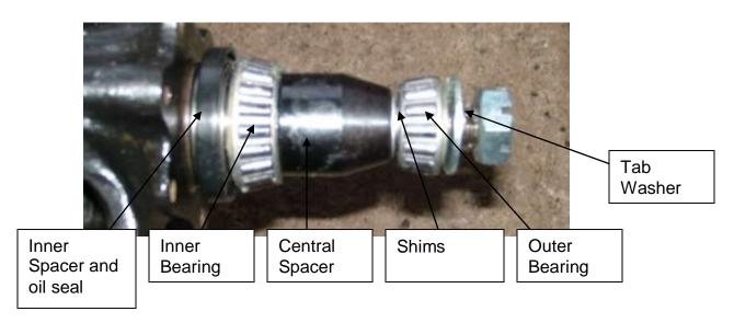
Once the bearing races are fitted I started the assembly. This is quite a fiddly job and many expletives were used. The first inner spacer needs to be slid onto the stub shaft. The black spacer then needs to be dropped in to the hub followed by the larger wheel bearing (pack the bearing with grease first). Then the oil seal can be tapped into the hub.
