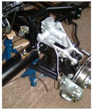
The last final job that I completed on this episode was fitting the clutch actuator kit which I got from Gerry. This was only a small job that took ages as I had to grind the bracket to suit where it fitted to the engine. It was probably made to fit a 302 engine and not a 289.
