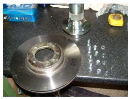
I thought I'd mate the hubs to the discs first, then I'd fit the bearings, spacers, shims and seals to the hubs.
