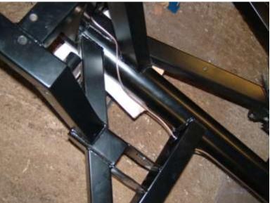
The main thing to remember is that the brake pipes need to be secured every 9 inches. P-clips are provided in the kit to suit the 3/16" pipe. There are a number of ways to fit the P-clips I just drilled the holes and tapped them to M4 and used bolts and washers to secure the clips.
