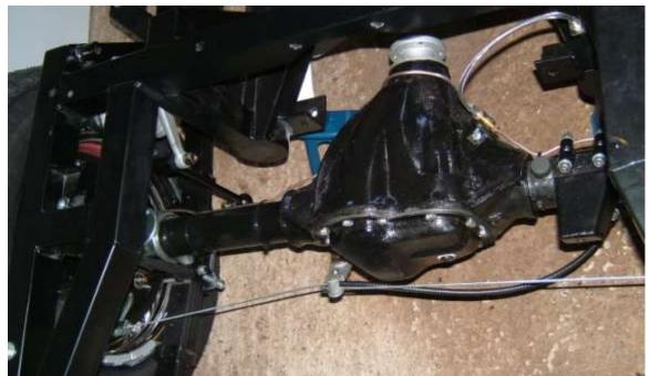
After a long wait the modified spring brackets arrived from the Gerry's fabricators. These brackets mount below the springs and connect to the shock absorber drop arms. The modification is to have two plates welded to them to accept the trailing arms (anti tramp bars). Unlike on the MGB, these are mounted upside down.
