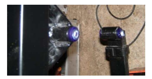
I came up with my own solution for the bump stops. The manual doesn't explain things that well and the mounting points that appear to be for the bumpstops would mean that the bump stops would impact on a round axle. I fitted the MGB crash stop plates with the Mini bumpstops mounted on them and this means that they would bottom out on a fairly substantial square section chassis member. I think that this was a much better solution (unless someone can advise otherwise.)
