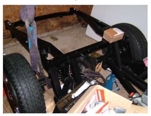
I then bolted the springs through the front eye to the chassis using the bolts provided in the kit. There are two possible holes that are used and it is the upper holes that are the correct ones. The lower holes are used for the anti tramp bars that will be fitted later.
