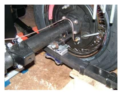
The bushes are then fitted to the rear eye on the spring and the rear chassis mount, smeared with the special poly bush lubricant and the standard MGB shackles are fitted and bolted up.
