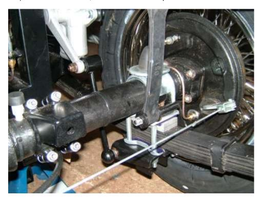
These brackets complete the sandwich around the rear leaf spring filling and it can be clearly seen where the drop links bolt to. Rear axle finished.
