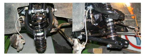
No bolts were tightened at this stage and the adjustable lower spring mount collar (which is used to adjust ride height) is at its lowest level. The king pin trunnion / hub / brake disk assembly can now be attached with the bolts and washers provided. I connected the bottom of the trunnion to the lower wishbones first and then the top to the top wishbones. There is a spacer tube that fits between the top wishbones.
