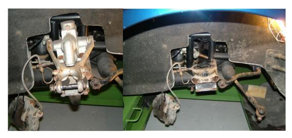
The lower wish bone pivot is retained as is the kingpin trunnion / hub assembly.
