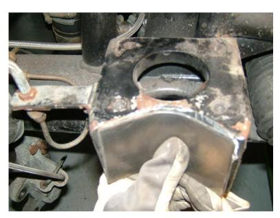
This needs to be welded in. It's not a structural weld and therefore can be tackled by most hobby welders. A good quality Arc or Mig set is perfect for mild steel. Before you commence, ensure the battery is disconnected from both terminals (positive and negative), make sure all combustible materials are removed from the vicinity and a bucket of water or fire extinguisher is available........
