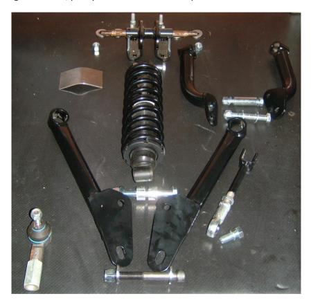
The only things needed, in addition to the parts shown above, are bushes. As two wishbone sets are used two equivalent MGB bush sets are needed. I've had good experience with poly bushes so I ordered two packs of these.
