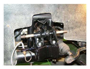
The wishbones can be fitted with the damper and spring. Copper slip was smeared on the top and bottom coils of the spring to prevent squeaking and also on threads as salt spray loves rotting unpainted mild steel and I may want to undo the nuts one day. Two of the lower wishbones have threaded bosses, these are fitted towards the front as the adjustable antiroll bar drop links attach to these. The galvanised spaces fit between the lower wishbones and the lower damper mount
