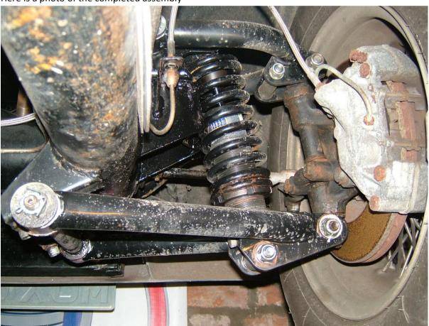
As already stated, I'd recommend that the bolts are not fully tightened until the suspension is loaded. This prevents the poly bushes from been strained which may result in premature failure. The torque settings to be used are a combination of those advised in the Hawk build manual and those advised in an MGB owner's manual.
