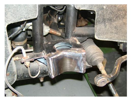
I used an arc welder and it can be seen from the blue marks on the plate that there's plenty of penetration meaning a good weld.
