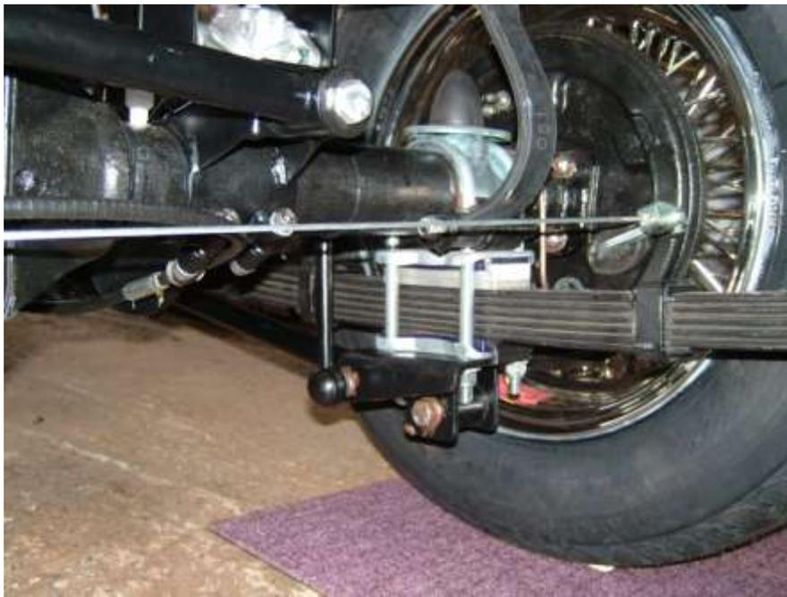
The panhard rod clamps onto the rear axle at one end and mounts to the chassis at the other. The aim with this is to get it close to horizontal. I planned to fit this loosely and then tighten it up when the chassis was fully loaded.
