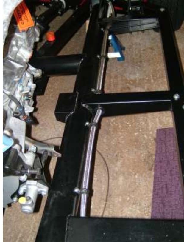
I bought some 16mm insulated stainless steel P clips to mount the fuel line. As with the brake lines, the fuel line needs to be secured every 9 inches along the vertical face of the chassis member. This is all that can be done on the fuel line at this stage as the fuel tank is situated within the boot and the final fit needs to be done when the body is back on.
