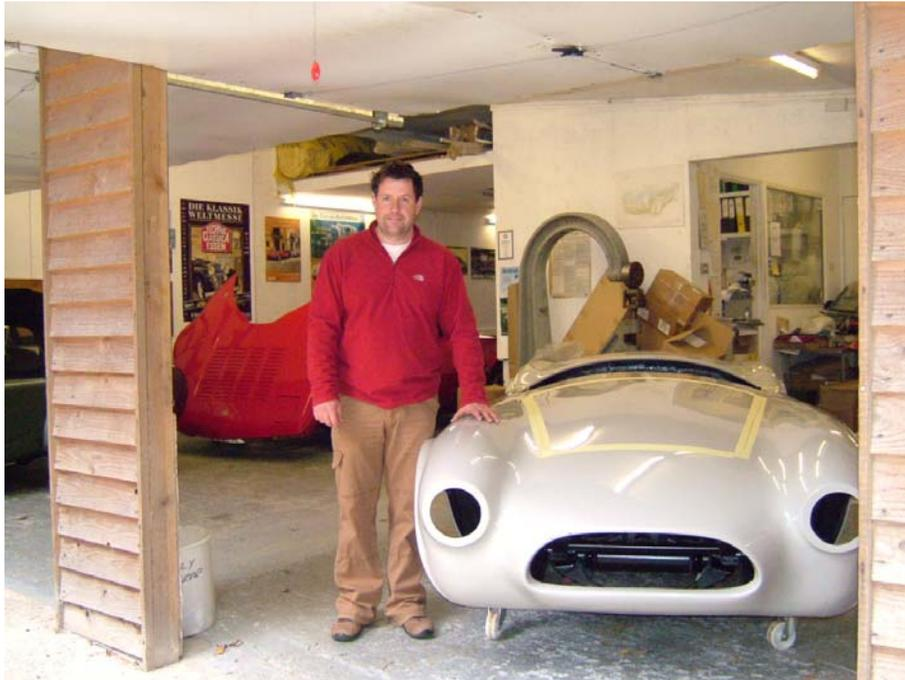
The body shell is fixed to the chassis and this is bolted to 2 transport bars that are mounted on castors. This makes it fairly easy to move around and once we are back at home I just need to unbolt the transport bars and ship them back.
