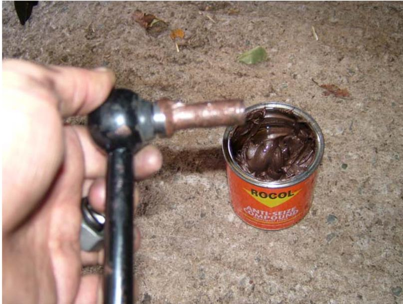
Next up, the Kingpins. Top trunion to the shock absorber first (with bushes well lubricated).
