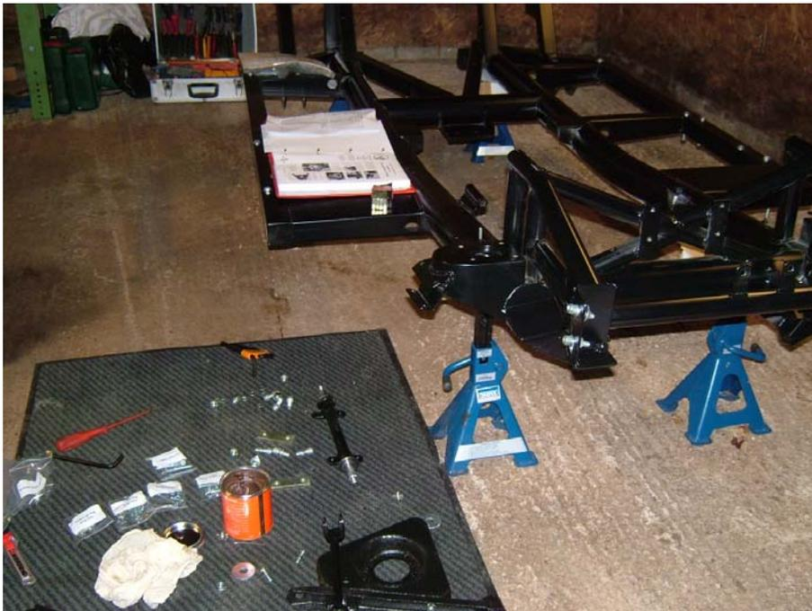
From my experience it's always good to do a dry run with nuts and bolts so you find out if they fit and also work out the correct order for washers (spring and flat). The other thing I decided to do, after stripping an MGB with all of its rusted nuts and bolts and after reading the Hawk build manual, was to use anti seize compound on all of the bolts. This can be a bit messy but I know it'll pay dividends in years to come.
