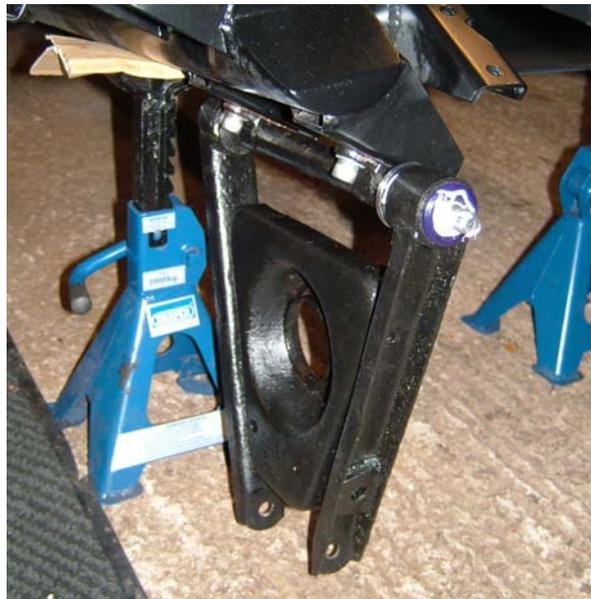
As you can see, I ensured that the bushes are well lubricated where they come into contact with metal (in this case the large counter washers that aren't included in the kit).
