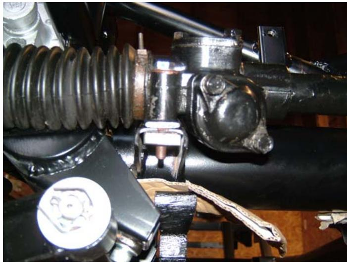
Use the bolts provided in the "Steering rack" bolt pack and some anti seize compound. The bolts pass through the steering rack, through the spacer, through the chassis and into the threaded plates.
