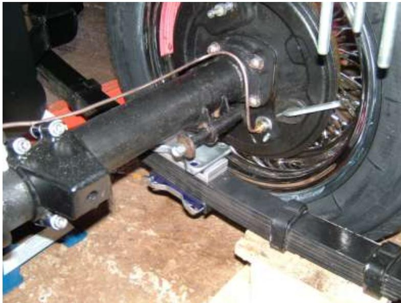
The bushes are then fitted to the rear eye on the spring and the rear chassis mount, smeared with the special poly bush lubricant and the standard MGB shackles are fitted and bolted up.
