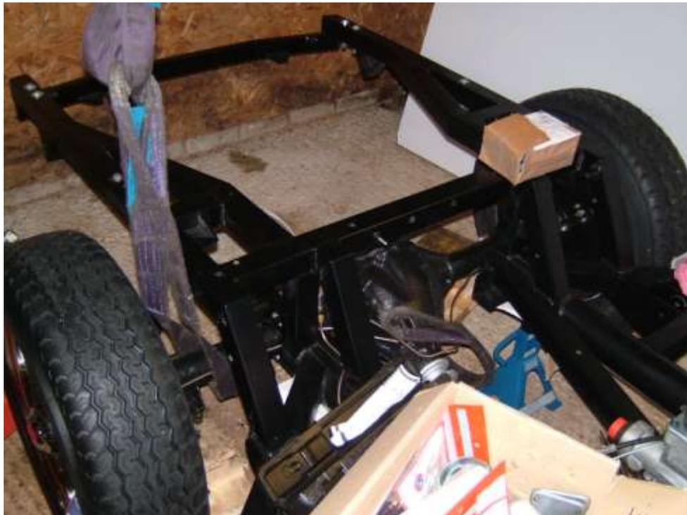
I then bolted the springs through the front eye to the chassis using the bolts provided in the kit. There are two possible holes that are used and it is the upper holes that are the correct ones. The lower holes are used for the anti tramp bars that will be fitted later.
